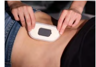
Fig. 1: Smart patch comprising a soft disposable part (white module) and an integrated sensor and AI analysis unit (grey module)
